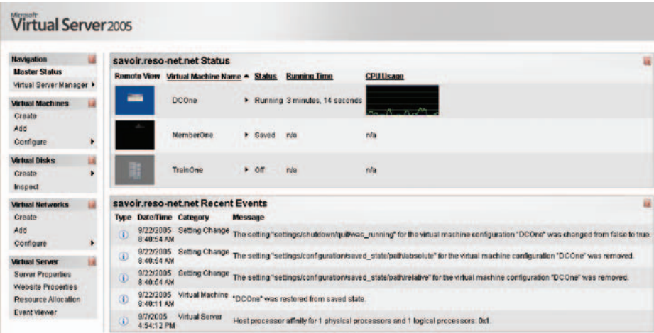
Figure 2: Using Virtual Server Virtual Server lets you operate several instances of an operating system within a physical server.
